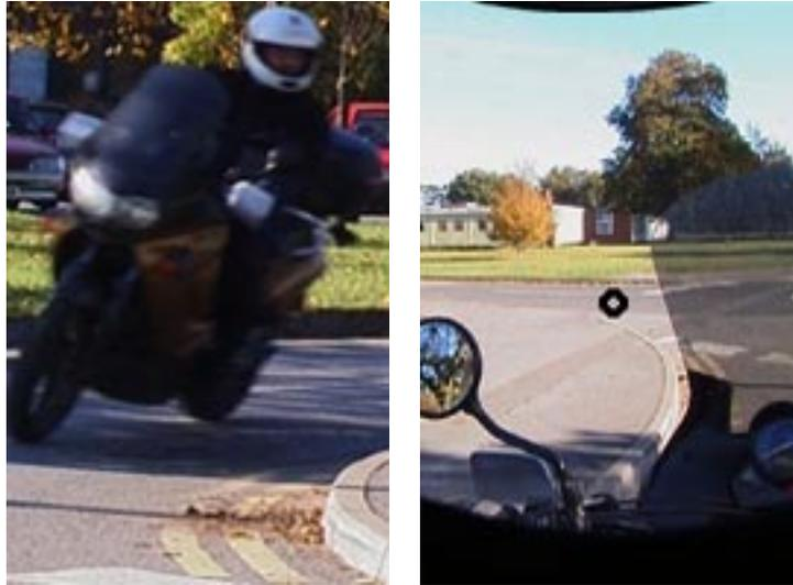
*Figure 4. Left Panel* - A motorcycle approaching a bend. Note the driver's head is offset from his locomotor axis supplying GAD information. *Right Panel* - The view from the motorcycle with the point of gaze marked as a black disc. In addition to the visual reference supplied by the windshield and mirror, the helmet both limits the field of view and supplies a visual reference that is fixed to the head angle not the locomotor axis.
