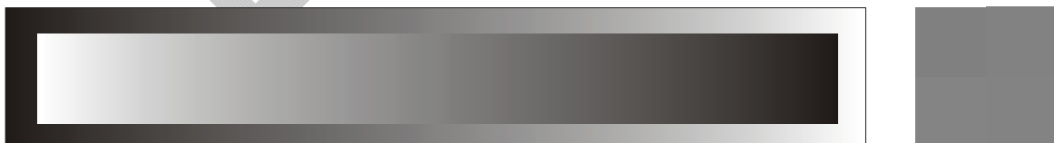
Figure 3.3: Perception of brightness. In the grey wedge on the left side, ranging from white to black (surrounded by a frame of opposite polarity) a human observer can discriminate approximately 5000 shades of grey, about 20 times more than the levels provided by a typical 8-bit image: boundaries between areas of a single unit difference ( 1/256 of range) are visible, as can be seen by close inspection of the set of four squares on the right.
