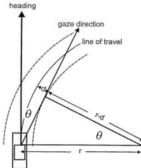
**Fig. 2** Geometry of tangent-point steering. The curvature of the bend ( $1/r$ ) can be obtained from the gaze angle  $\theta$ , using the geometry of the right angled triangle. Here,  $\cos\theta = (r-d)/r$ , where  $d$  is the distance of the driver from the lane-edge. However, the expansion of the cosine gives  $\cos\theta \approx 1 - \theta^2/2$ . Substitution for  $\cos\theta$  then gives:  $1/r \approx \theta^2/2d$
